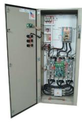
The RX2E / RX3E Enclosed Combination Soft Starter is a rugged, simple to use soft starter with built-in motor protection, providing greater control in starting and stopping of three phase motors. RX2E / RX3E Series Enclosed Combination Soft Starters come standard with a circuit breaker, full voltage rated emergency bypass contactor, door mounted Start/Stop push buttons, Local/Off/Remote selector switch and door mounted keypad.
