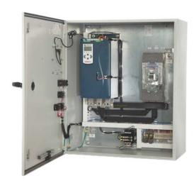
Benshaw MX4PB Packaged Soft Starters provide solid state reduced voltage starting for normal operation and full voltage emergency backup starting with complete electronic motor protection at the flip of a switch. The unique, dual redundant design of our MX4PB Series soft starter is ideal for standard and heavy duty soft start applications where downtime is extremely disruptive to production operations and cannot be tolerated.
